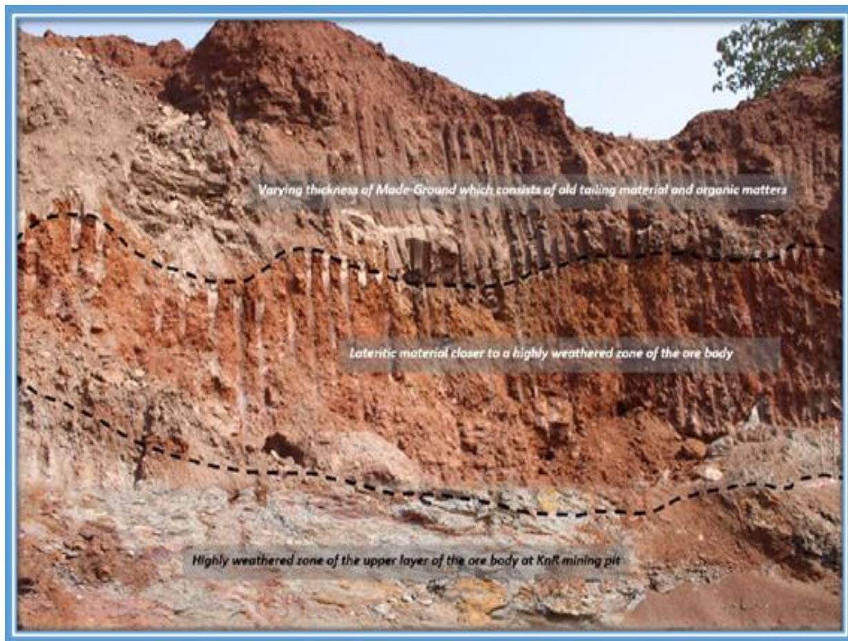
Figure 4- 13: An Exposed Active Mining Dig Face at KnR Pit Shows Different Soil Layers.
