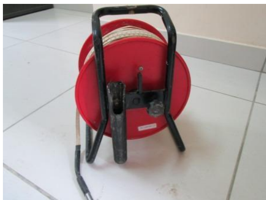
Figure 5.14-5: Dip Meter with Sensor
