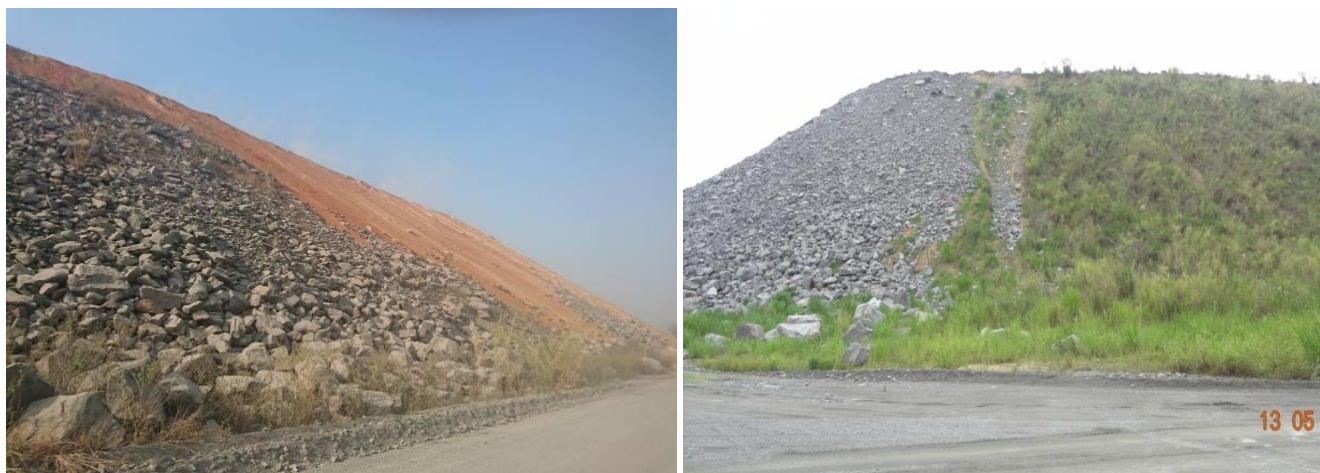
Figure 2.3-5: Waste Rock Stockpiles Layered with Laterite and Re-vegetated
