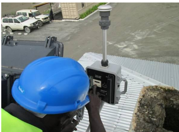
Figure 5.14-3: Installation of Tactical Air Sampler at Charlie 4 Gate
